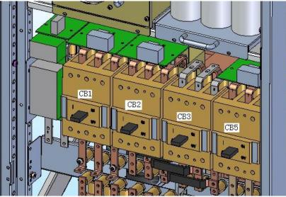
The UPS unit circuit breakers are CB1, CB2, CB3 and CB5.
